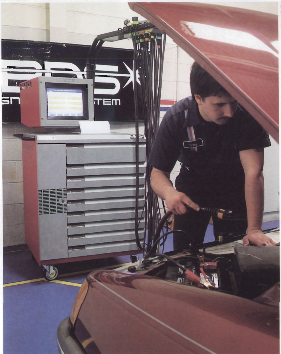
AMSO helped Ford develop the Service Bay Diagnostic System—a new generation of diagnostic equipment which is faster and more accurate than previous methods.
