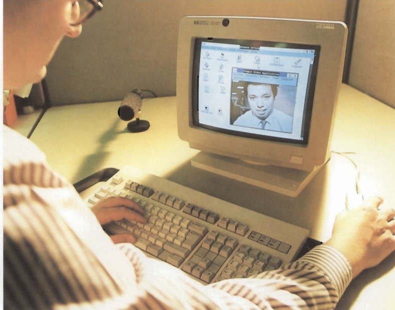
Stephen Gale and Colin Baker (on screen) can see and hear each other while they share data on this prototype system developed at HP Labs Bristol.
