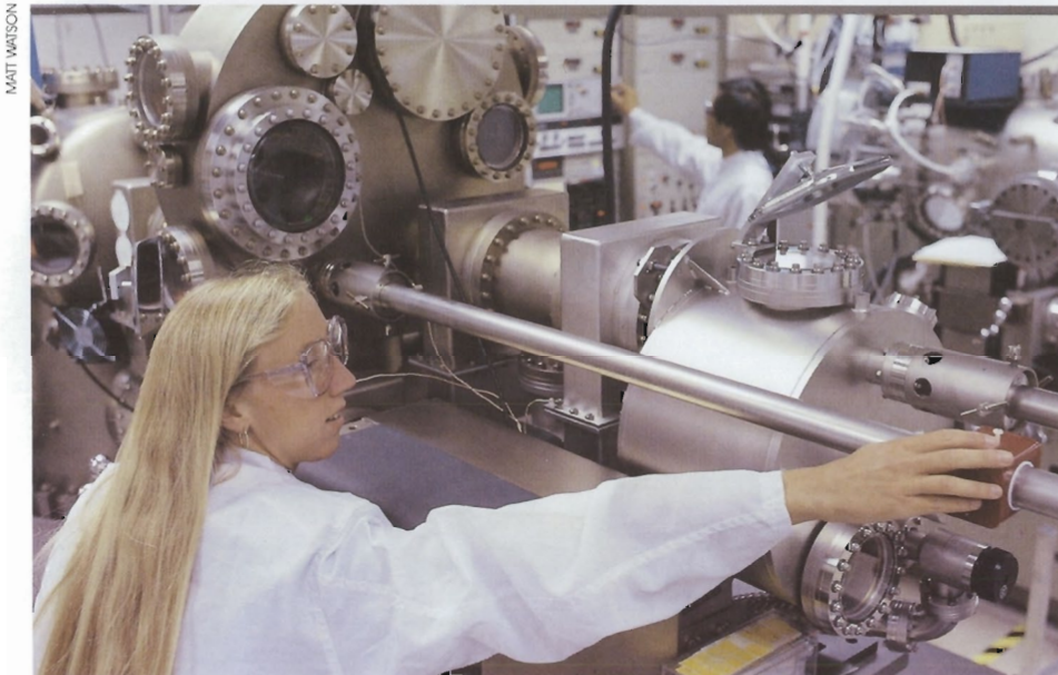
HP Labs researcher Alice Fischer-Colbrie uses a molecular-beam epitaxy machine to deposit gallium arsenide—atomic layer by atomic layer—to develop transistors, integrated circuits and optical devices.
